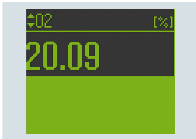
Local user interface (LUI) of SITRANS SL in the detector unit (display of measured value)
