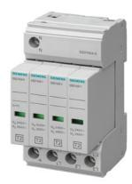
Surge arrester Type 2 Requirement class C, UC 350V Pluggable protective modules 4-pole, 3+1 circuit for TN-S and TT systems Narrow design
