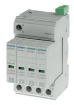
Surge arrester T2, UN 240/400 V, UC 350/264 V AC, pluggable protective module, 3+1 circuit (TN-S, TT), Width 49.2 mm
