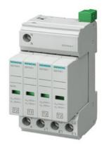
Surge arrester Type 2 Requirement class C, UC 350V Pluggable protective modules 4-pole, 3+1 circuit for TN-S and TT systems with FRN display, narrow type of construction
