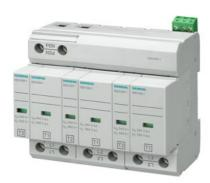
Combination arrester type 1+2 Requirement class B+C, UC 350V Pluggable protective modules 3-pole, 3+0 circuit for TNC systems with remote display
