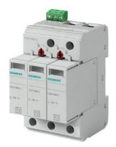
Surge arrester, Type 2, pluggable protective modules, UC 750V AC, 3-pole, for 4-wire networks (L1, L2, L3, pen), with remote signaling
