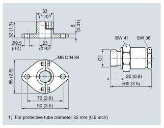
Mounting flange to DIN 43734 (left) and threaded sleeve (right) for installing straight thermocouples, dimensions in mm (inches)
