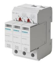
surge arrester T1/T2, UC 1050V DC, Imax 40 kA Short-circuit strength 80 A, 2+V circuit, for isolated and grounded PV systems
