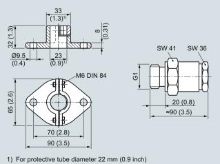
Mounting flange to DIN 43734 (left) and threaded sleeve (right) for installing straight thermocouples, dimensions in mm (inches)
