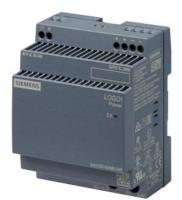
SIPLUS LOGO! Power 24V 4A for medial stress -40...+70°C start up at -25°C based on 6EP3333-6SB00-0AY0 . stabilized power supply input: 100-240 V AC output: 24 V / 1.3 A DC
