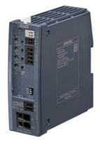
SITOP SEL1400 10 A Selectivity module 4-channel with limiting characteristic Input: 24 V DC/40 A Output: 24 V DC/4x 10 A Threshold value adjustable 2-10 A With monitoring interface
