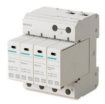
Lightning conductor T1/T2, UN 240/400 V, UC 335/264 V A.C., pluggable protective modules, 3+1 circuit (TN-S, TT), Width 72 mm
