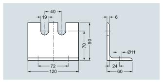
Mounting bracket 7MF9004-6AA (M13), dimensions in mm
