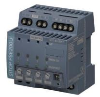
SITOP PSE200U 3 A Selectivity module 4-channel input: DC 24 V/12 A output: 24 V DC/4x 3 A Level adjustable 0.5-3 A mit status message for each output
