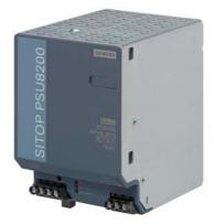
SITOP PSU8200 20 A Stabilized power supply input: 120-230 V AC 110-220 V DC output: 24 V DC/20 A
