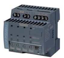
SITOP PSE200U 3 A NEC CLASS 2 Selectivity module 4channel input: DC 24 V/12 A output: 24 V/4x 3A NEC class 2 Level adjustable 0.5-3 A with common signaling contact
