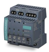
SIPLUS PS PSE200U 3A with conformal coating based on 6EP1961-2BA31 . Selectivity module 4-channel input: 24 V DC output: 24 V DC/3 A per channel Output current adjustable 0.5-3 with status message per channel
