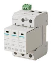
Lightning conductor T1/T2, UN 240/400 V, UC 335 V A.C., pluggable protective modules, 3+0 circuit (TN-C), Width 54 mm with remote signaling
