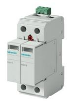
Surge arrester, Type 2, pluggable protective modules, UC 800 V AC, 1-pole, Varistor connected in series and gas-filled spark gap with remote signaling
