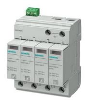
Surge arrester Type 2 Requirement class C, UC 350V Pluggable protective modules 4-pole, 3+1 circuit for TN-S and TT systems with remote display
