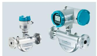
The complete flowmeter system SITRANS FC consist of a new FCS400 sensor in sizes DN 15 to DN50 mm and a FCT030 multichannel/multifunctional in compact or remote versions, or a single Modbus-channel FCT010 transmitter in compact version. The flowmeter is based on the latest developments within digital signal processing technology – engineered for high measuring performance:
