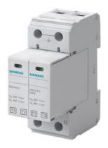
Lightning arrester type 1, 12.5 kA, lightning protection class III and IV, for 3-wire networks (L, N, PE), UC 335V/264V AC (L-N/N-PE), Mechanical defect indication
