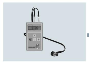
The thickness gauge is used to measure the wall thickness of the pipe that a clamp-on ultrasonic flowmeter is installed on. The wall thickness value is a vital factor in the flow computation model and a prerequisite for precise clamp-on ultrasonic flow measurement. When measuring any pipe wall thickness the thickness gauge can also be used as a stand-alone tool used to measure the wall thickness of any metallic or non-metallic pipe materials capable of acting as an ultrasonic wave conductor.
